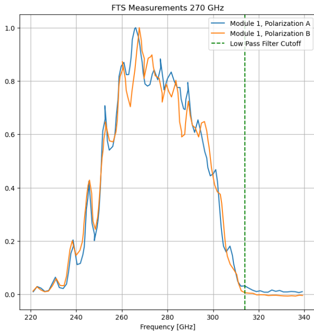
Fig. 8. The peak-normalized mean passbands of both polarizations for the one module 270 GHz module measured in lab.
